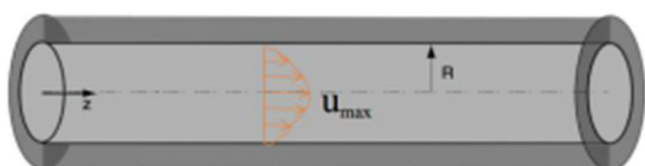
Figure 2. Schematic diagram of laminar flow through a needle
